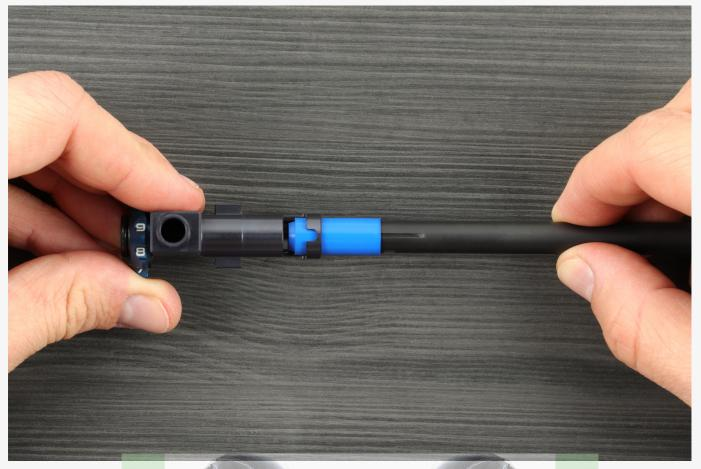
12. In the final stage, make sure the bucking does not chafe against the tensioner window. If you are unable to get the barrel into place, carefully lubricate the bucking again and try once more. If the problem persists, try using other hop-up bucking because this one is too large in diameter.
