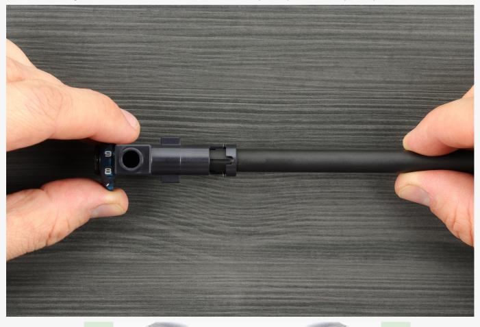
14. Install the barrel latch (this may require gently moving the barrel back and forth)—for bucking with a longer flange, (such as Maple Leaf) use a latch with a longitudinal incision.
