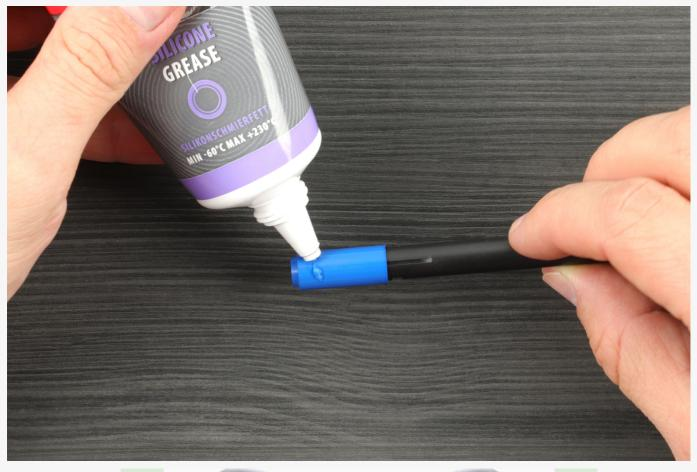
10. Spread the grease on the outer surface with your fingers, leaving a thin layer of grease.
