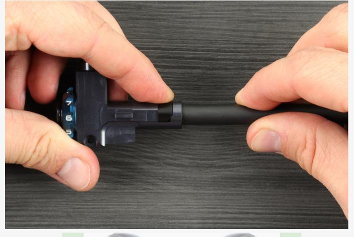
16. Install the barrel sleeve.
