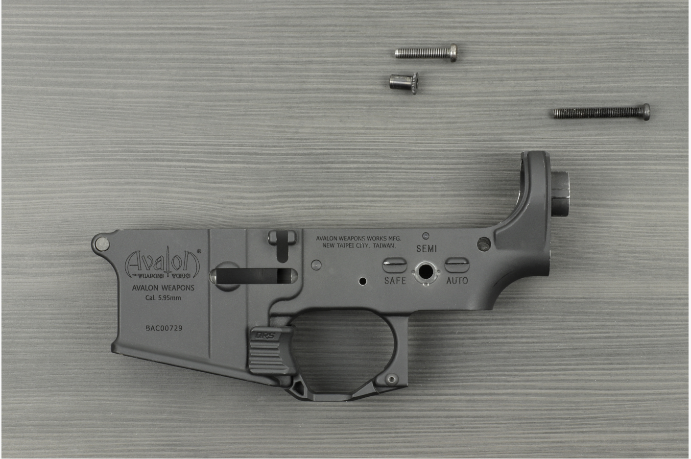
Option 2 - Use of a flat screw to stabilize the spring guide
