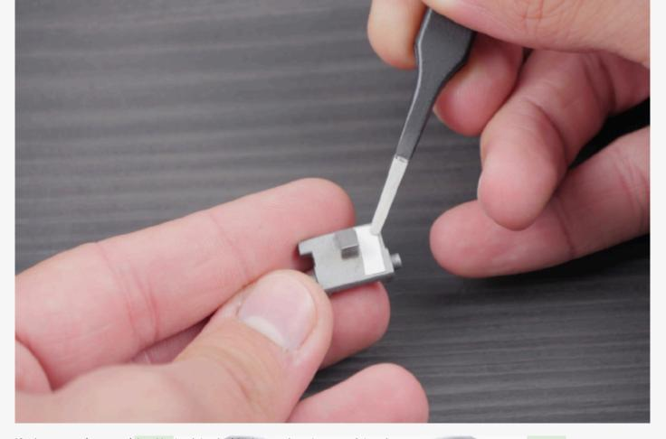
19. Place one trigger anti-backlash sticker inside the moving element of the trigger.
