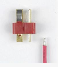
25. Have a look at the connection and check if it is done properly. Pay attention while soldering – it should fill the soldered space correctly and the solder cannot be oxidized. Remove excess rosin from the connection.
