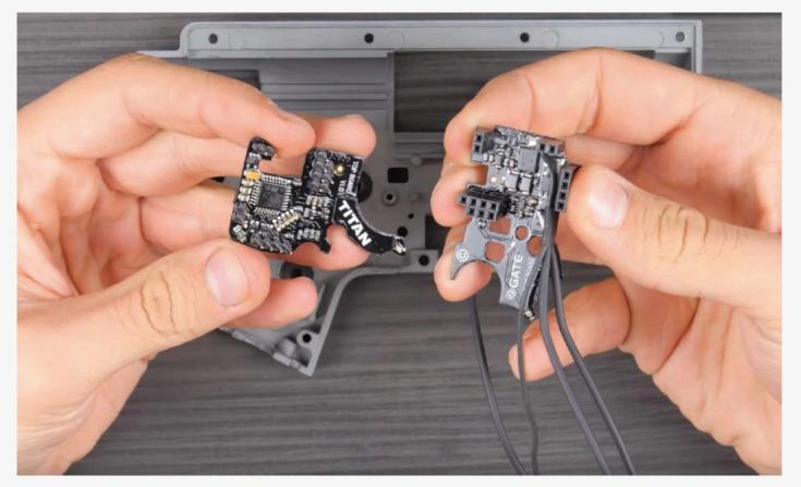
6. Place the bottom board in the bottom part of the gearbox. Do not use a screw yet. Check if the bottom board is laid flat in the gearbox.
